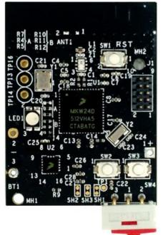
Figure 1. IoT Low Power Sensor Node reference design board
