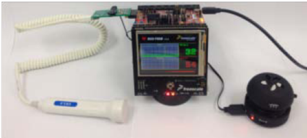
Figure 5-2. System's hardware working with K53N512 microcontroller
