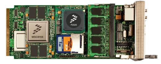
The MSC8156 DSP delivers a high level of performance and integration, combining six fully programmable, SC3850 DSP cores, each running at 1 GHz. This 6 GHz of processing power, coupled with an architecture highly optimized for wireless infrastructure applications, make this an ideal device for developing solutions for the next generation of wireless standards.
