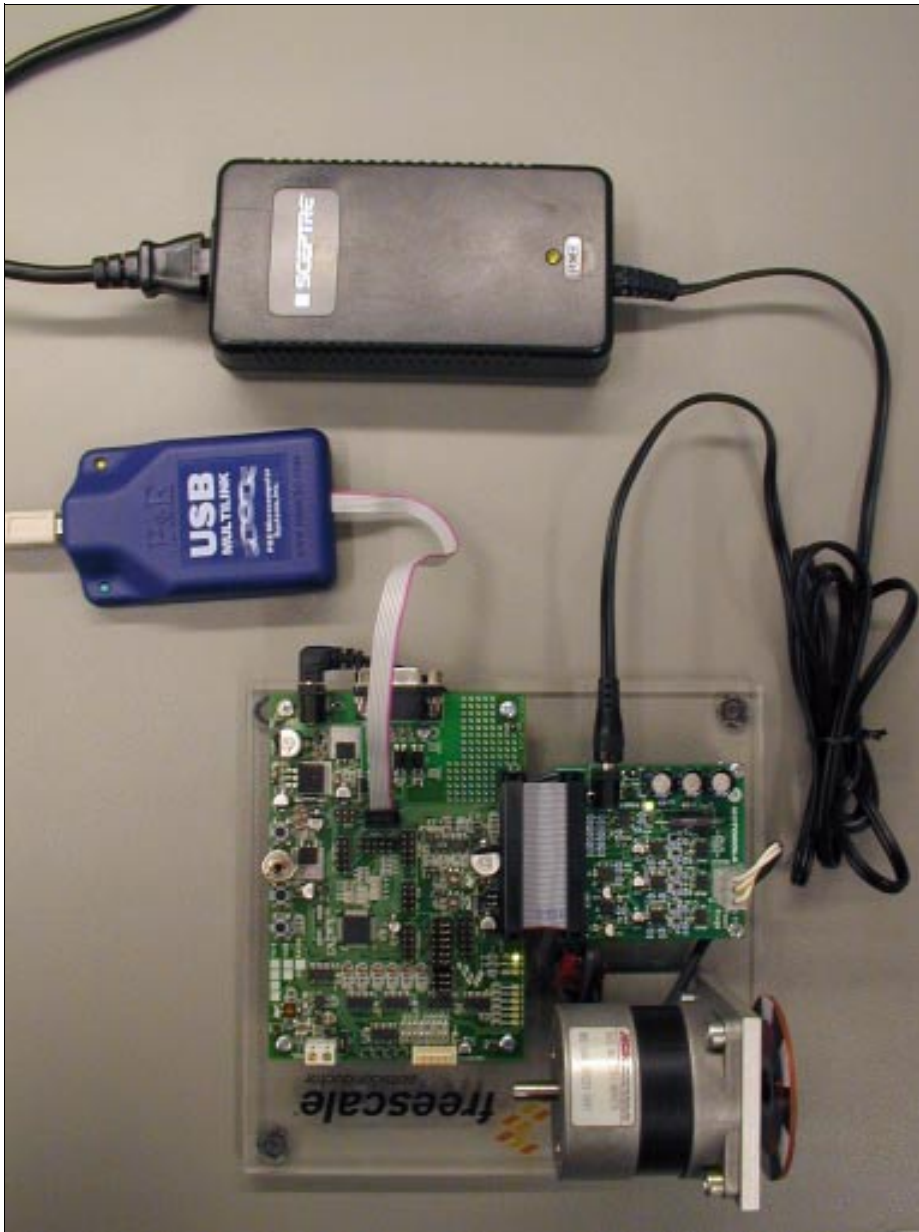
Figure 6-2. Sensorless BLDC Demo Setup
