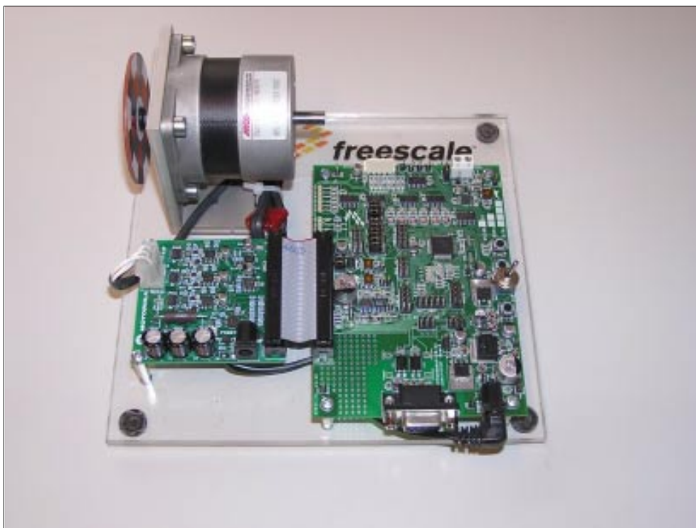
Figure 1-1. Sensorless 3-Phase BLDC Motor Demo Using MC9S08AW60
