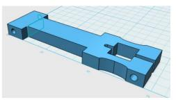
A new encoder-holder was also printed, to better fix the sensor and reduce the shifting during the race.
