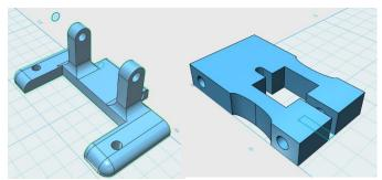
The led board has been detached from the camera board and installed with a different support to the stick. This was done to give more mobility to the led board and to have a better orientation of the light.
