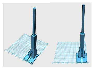
With it, a new camera holder, the piece that attach the camera board to the stick, was adapted and printed.
