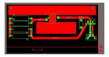
The LED is mounted one a PCB circuit too. To feed it with the right voltage, a voltage regulator is needed: the Texas Instrument 7805 Positive Voltage Regulator.
