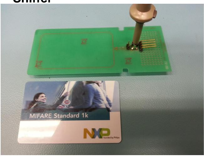
Single turn coil, connected to high impedance scope probe
