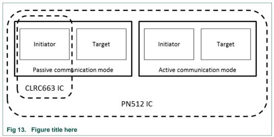
The PN512 reader IC supports all possible NFCIP-1 configurations whereas CLRC663 reader IC only provides support for Passive Initiator configuration.
