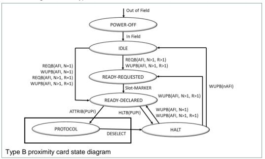
When the card is out of the RF field generated by the reader IC, it is in the POWER-OFF state. As soon as it is powered, it enters the IDLE state, where it waits for REQB or
