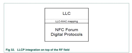
Two LLCP components exchange information in the form of LLC Protocol Data Units (PDU). LLC PDUs exchange either LLC management data units such as CONNECT PDU and DISC PDU or upper layer information encapsulated in I PDU and UI PDU.
