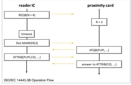
As we said before, the value of R is randomly chosen by the card, and shall always be between 1 and N. As we can see in the figure above, the Slot-Marker commands do not need to be called sequentially with incremental slot numbers.
