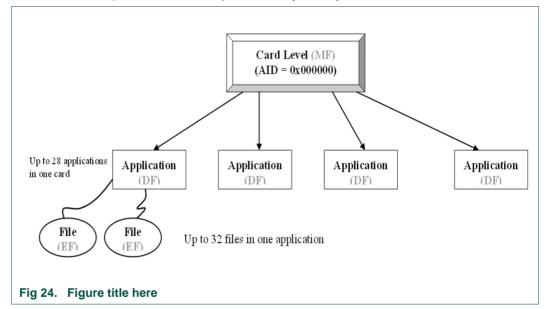
A file can only be selected after the dedicated application where it is hold has been selected. Once within the application, files can be accessed using the files' IDs. Five different types of files can be created within each application:
