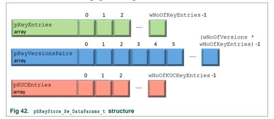
The elements of these arrays are structure variables, which are described in the following lines.
