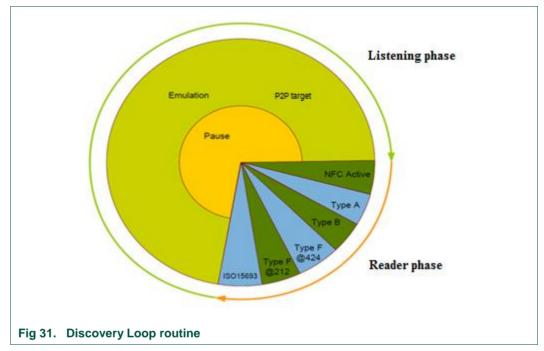
Unlike HAL, the Discovery Loop uses MCU timers for measuring the guard times, instead of the reader IC timers. Due to the fact the OSAL layer does not provide any thread creation capabilities, the Discovery Loop can only run in the main thread called from the upper application without any possibility of interruption, therefore the upper application is blocked until the Discovery Loop routine exits.
