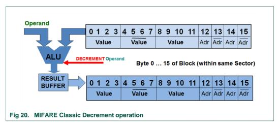
In case of loss of energy during one transaction, the value stored in the volatile memory will not be accessible anymore.
