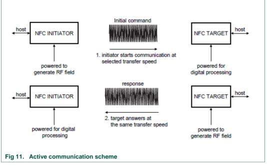
The main advantage of implementing the active communication, compared to the passive communication, is the larger coverage distance in case of the same bit rate, or the higher bit rate in case of the same coverage distance. According to the ISO/IEC 18092 standard, higher bit rates than 424 kbps are expected for this communicating mode in future standard updates.
