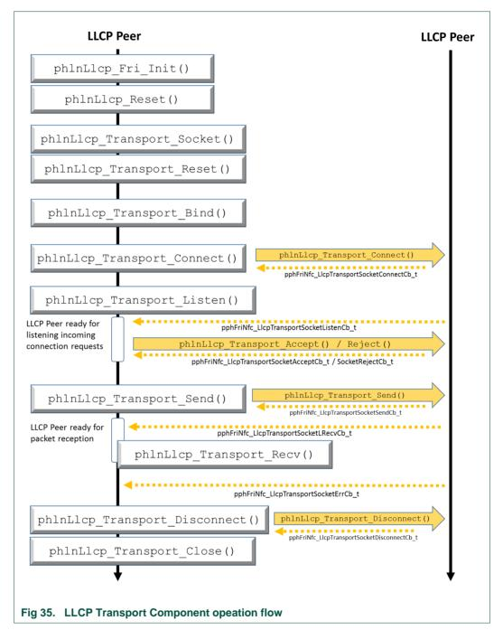
As it is explained in detail in the LLCP Transport API section (see section 7.1.5.2), some of the functions that are described here should not be directly called by the developer since they are called internally by upper layer components such as the SNEP protocol.
