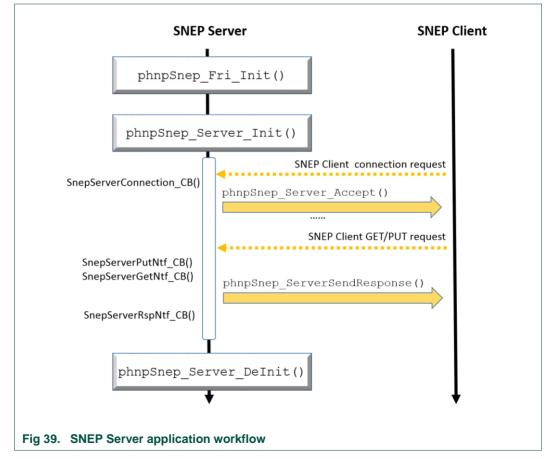
A SNEP Server in the listening phase is capable of accepting SNEP Client requests. The connection establishment and the data exchange generate notification events which trigger callback functions. More information of the SNEP Server callback functions is available in Section 7.2.3.3. The SNEP Server API functions are detailed here following:
