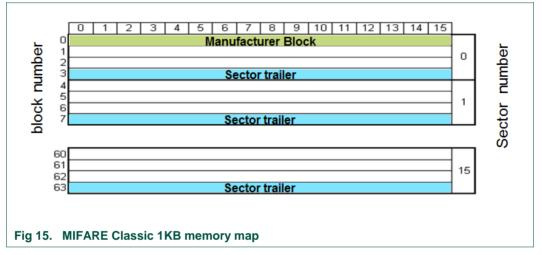
Block 0 of sector 0 is called the Manufacturer Block and contains the IC manufacturer data. This block is programmed during production and it cannot be changed afterwards.
