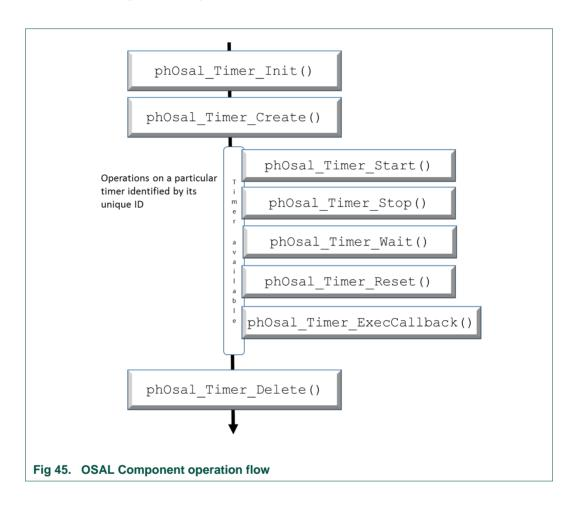
The following figure depicts the flow of functions to be called in order to ensure the correct functioning and management of hardware timers.
