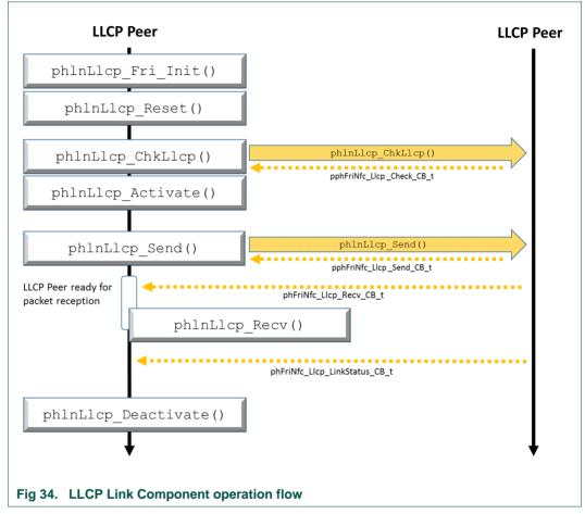
As it is explained in detail in the LLCP Link API section (see section 7.1.4.2), some of the functions that are depicted in this flow should not be directly called by developers since they are internally called by upper layer components such as the LLCP Transport component.
