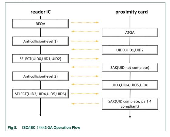
An example of an initialization dialog between a reader and a Type A card with a 7 bytes UID is shown below:
