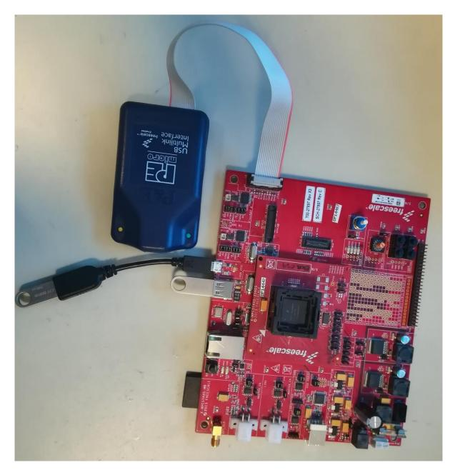
To load the software on the mainboard, one would need an USB Multilink Interface or a Lauterbach debugger.
