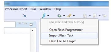
• Select the target task to switch mcu mode: MPC5643L\_DPM\_VLE to switch from LSM to DPM MPC5643L\_LSM\_VLE to switch from DPM to LSM
