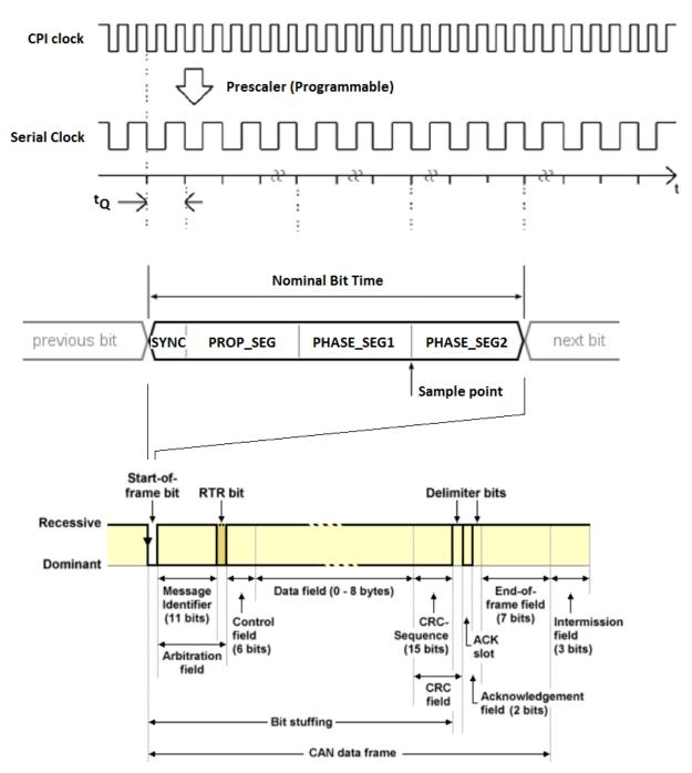
Starting from a data frame transferred on the bus. A desired baudrate tells how many bits are sent on the network per second. The Nominal Bit Rate (baudrate) is uniform throughout the network and is given by:
