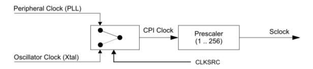
The clock source selection is done by the CLK\_SRC bit of the CTRL register. Moreover this register contains other fields used to control bit timing parameters as was mentioned above: PRESDIV, PROPSEG, PSEG1, PSEG2 and RJW. The SMP specifies if one or three samples per bit is used.
