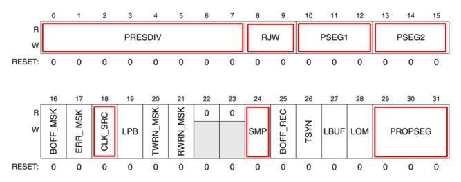
These parameters have to be properly calculated/selected to meet the CAN specification.
