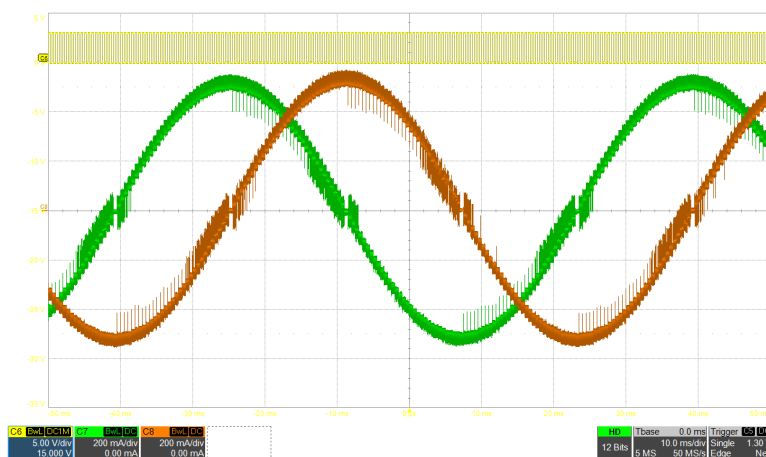
Figure 8-5. 1/32 Microstepping With smart tune Ripple Control Decay
