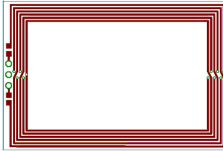
Fig 37. MFRC52x/PN51x/PN53x evaluation board antenna
