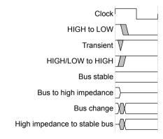
Figure 1 Key to timing diagram conventions
