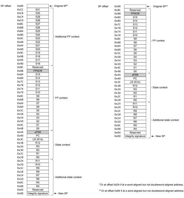
Stack frame for Secure floating-point state when FPCCR.TS = 1
