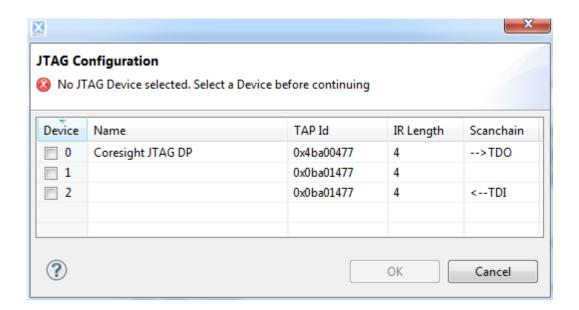
Device 1 is the M0SUB core. The device closest to TDI (device 2 here) is then the M0APP core. Make sure that you select the correct core for each debug connection!
