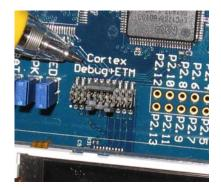
20 Pin Cortex Debug+ETM connector
