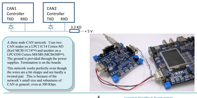
CAN: Controller Area Network Lab using NXP LPC Cortex-M processors.
