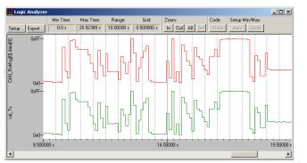
this in one of the bad spots and this is why the graph has the sharp jumps. This was confirmed with a CAN analyzer attached to the bus and an oscilloscope on the pot.
