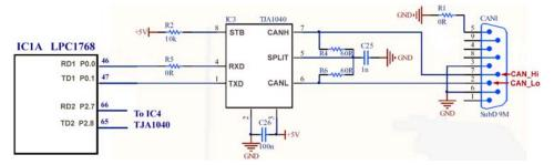
STB on IC3 when high disables the Transceiver. This is useful for low power modes or when the CAN controller is in Busoff mode. This will effectively remove the node from the bus. **TIP:** You need to use external hardware to set/unset STB.
