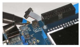
10 Pin Cortex Debug beside the legacy 20 pin JTAG Note the 10 pin cable end in the background.
