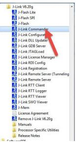
3. Typing the "connect" to connect the device, then type "device LPC54608J512", select the SWD by type "S" or select JTAG interface by "J". Next, set the speed: 4000 kHz.
