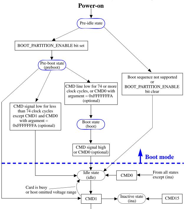
Figure 19 — MultiMediaCard state diagram (boot mode)
