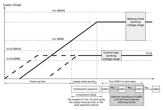
Figure 51 — eMMC power-up diagram
