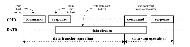
Figure 6 — Sequential read operation
