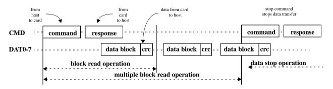
Figure 7 — Multiple-block read operation
