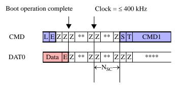
Figure 42 — Bus mode change timing (push-pull to open-drain)
