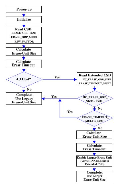
Figure A.15 — Erase-unit size selection flow
