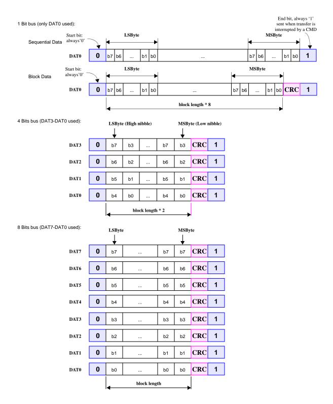
Figure 13 — Data packet format
