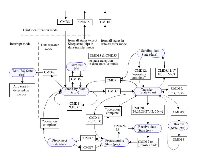
Figure 22 — MultiMediaCard state diagram (data transfer mode)
