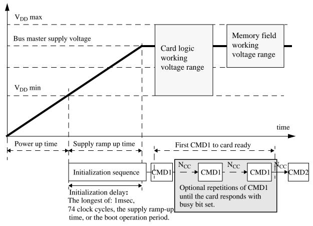
Figure 50 — Power-up diagram
