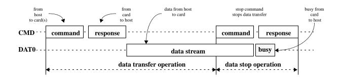
Figure 8 — Sequential write operation
