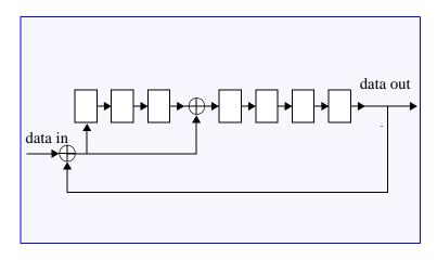
Figure 45 — CRC7 generator/checker
