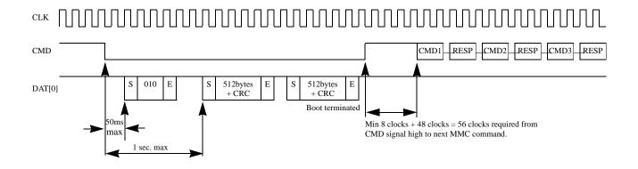
Figure 17 — MultiMediaCard state diagram (boot mode)
