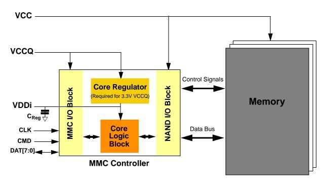
Figure 54 — eMMC internal power diagram
