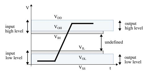
Figure 55 — Bus signal levels
