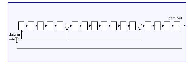
Figure 46 — CRC16 generator/checker
