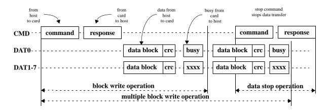
Figure 9 — (Multiple) Block write operation
