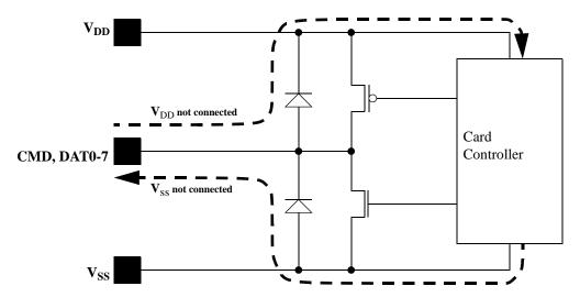
Figure 48 — Improper power supply
