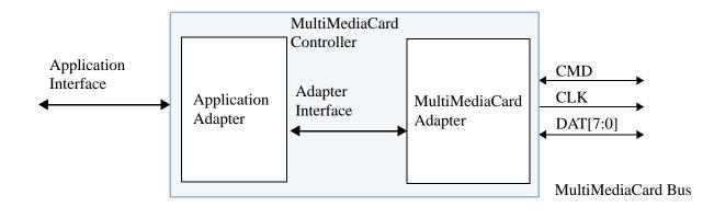
Figure 14 — MultiMediaCard controller scheme
