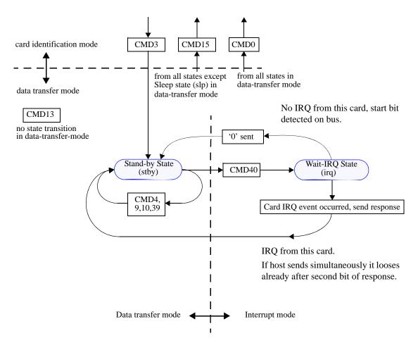
Figure 21 — MultiMediaCard state transition diagram, interrupt mode
