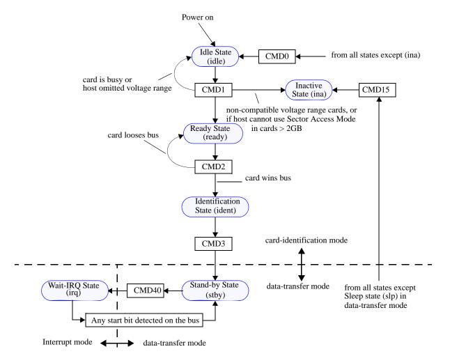
Figure 20 — MultiMediaCard state diagram (card identification mode)
