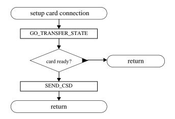
Figure A.6 — CIM\_SETUP\_CARD
