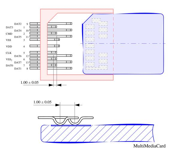
Figure A.2 — Modified MultiMediaCard connector for hot insertion
