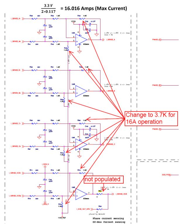
In case the board maximum current scale is increased to 16Amps and original shunts (current measurement resistors) are not updated as well, then there is a high risk of board damaging / burning.
