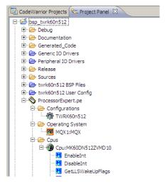
• Right click the CPU and select "Inspector". The CPU Component Inspector opens.
