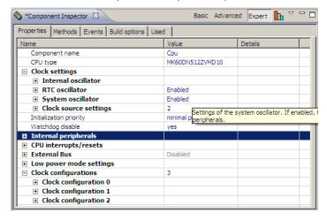
• Unfold the "Internal oscillator" item and set the required parameters.
