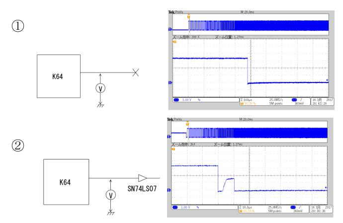
\*Power-supply voltage of SN74LS07 is 5V.
