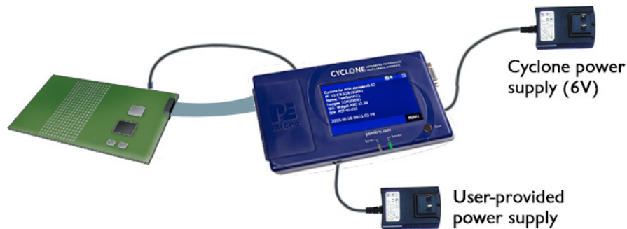
Figure 3-16: Via Power In and Power Out Jacks of Cyclone
