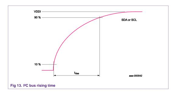
The I<sup>2</sup>C standard requires a  $t_{rise}$  time lower than 300 ns for 400 kHz and 1000 ns for 100 kHz.
