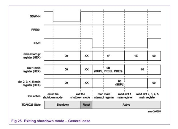
Exiting the shutdown mode, the sequence of event is exactly the same as before, as the state of the TDA8026 is the same after the reset sequence.
