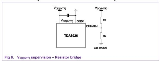
In this case PORADJ =  $V_{DD(INTF)}$ .R2/(R1+R2) and  $V_{DD(INTF)}$  is monitored indirectly: the TDA8026 enters the reset mode when  $V_{DD(INTF)}$ .R2/(R1 + R2) falls below Vbg.
