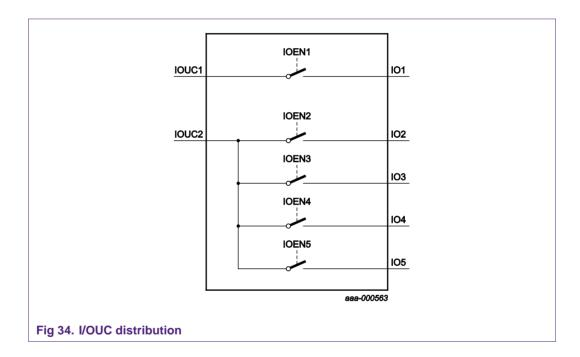
When more than one slot is activated at the same time, the host must always take care to activate only one I/O line at the same time. If not, a conflict will occur when two cards will receive the same command and try to answer on the same line, as shown in Fig 35.
