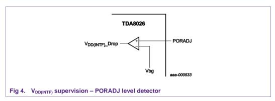
The TDA8026 compares the pin voltage level on pin PORADJ to an internal voltage reference called Vbg.
