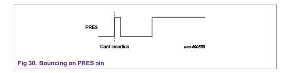
This could cause three interrupts sent to the host by the TDA8026. Some microcontrollers do not support this behavior.
