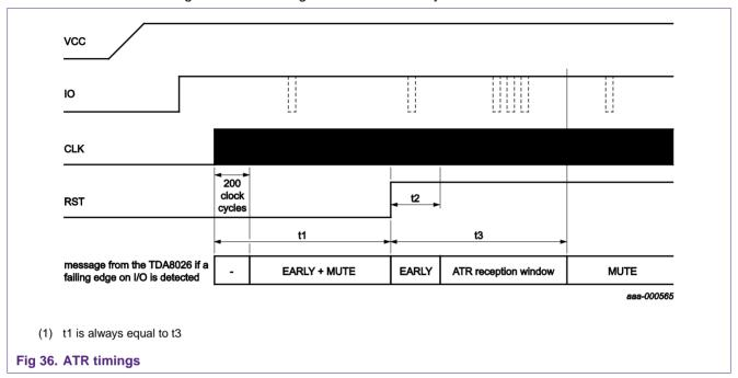
When a delay is not within the specification, the TDA8026 does not deactivate the card but send an interrupt and set its corresponding bit.
