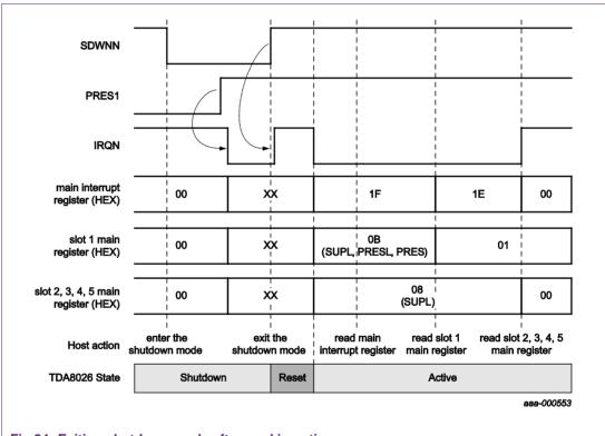
Fig 24. Exiting shutdown mode after card insertion
