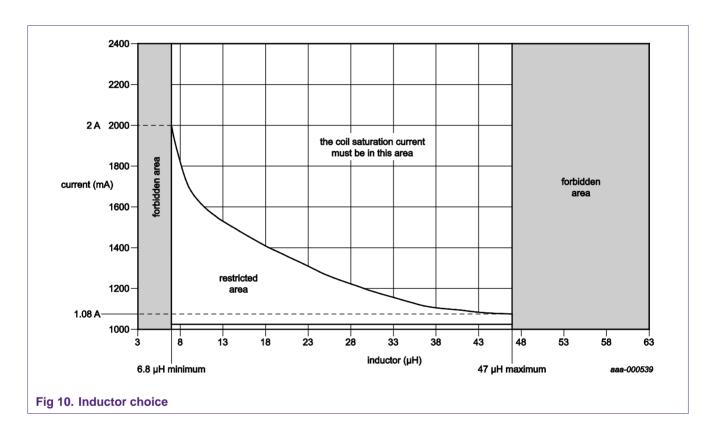
The chosen inductor must respect this requirement: the saturation current which induces 30% inductance drop must be above the limit value.
