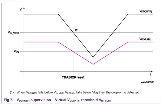
The resistor bridge is needed only in the case a specific threshold on  $V_{DD(INTF)}$  must be chosen for the application, but in the general case,  $V_{DD(INTF)}$  can be input directly on PORADJ.
