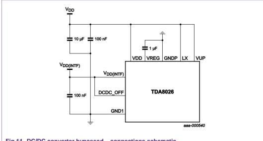
Fig 11. DC/DC converter bypassed – connections schematic
