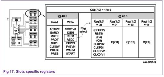
When there is a communication at address 42h, the accessed register is defined by the REG[1:0] value stored at address 40h.
