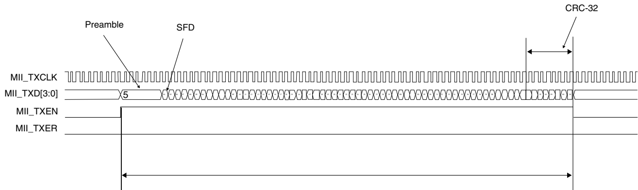
Figure 45-122. MII transmit operation
