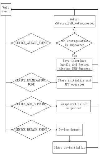
Figure 42 Enumeration and detachment flow
