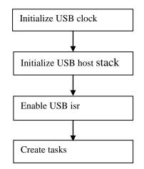
Figure 43 Main application function flow
