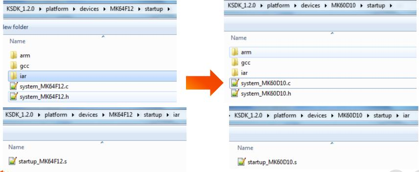
Other driver/hal/system device specific files should be created, for example, under path sdk\_install\_folder\platform\system\src\clock\, each device has its own clock definition files, Copy \MK64F12 to \MK60D10 and modify these files for K60D10.
