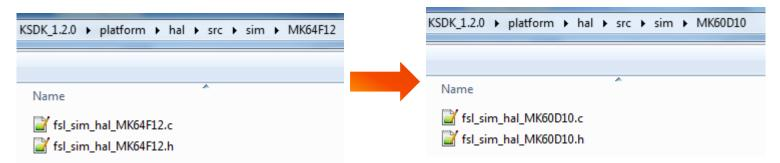
Then add SIM content of K60D10 into common file "fsl\_sim\_hal.h" which is located at sdk\_install\_folder\platform\hal\inc
