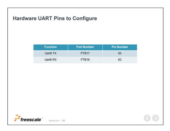
Here are the pins we need to deal with for the UART. This uart is connected to the debug interface chip on this board, and it allows for the uart to print on the PC terminal window.
