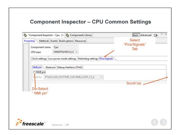
Since our project does not require an nmi interrupt routine, we will uncheck this box. Also, if you are using the nmi pin as a signal pin, like the FRDM board.
