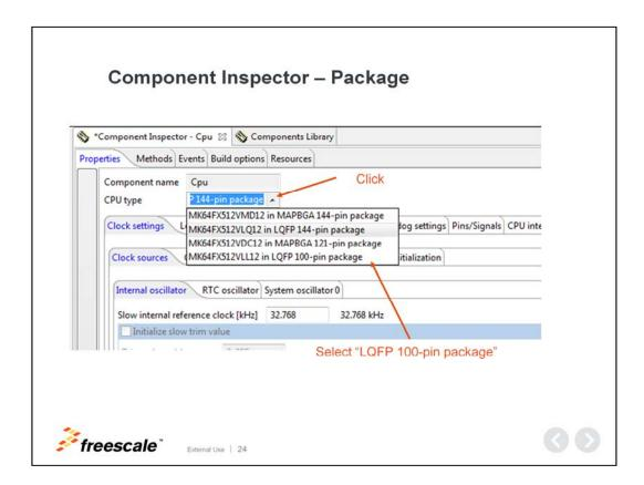
Selecting the "package" of the chip. Remember that each chip has several packages, selecting the proper package here is vitally important to have the proper pin muxing.
