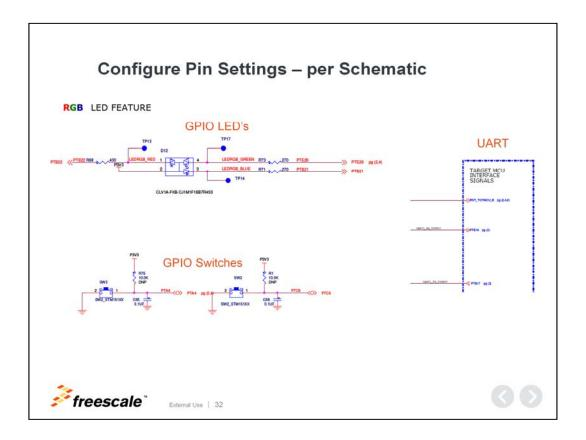
Now we move into the pin settings. And our io's will be: LED's are on ports PTB-21, PTB-22, and PTE-26 SWitches are on ports PTA-4, and PTC-6 UART is on PTB-16, and PTB-17
