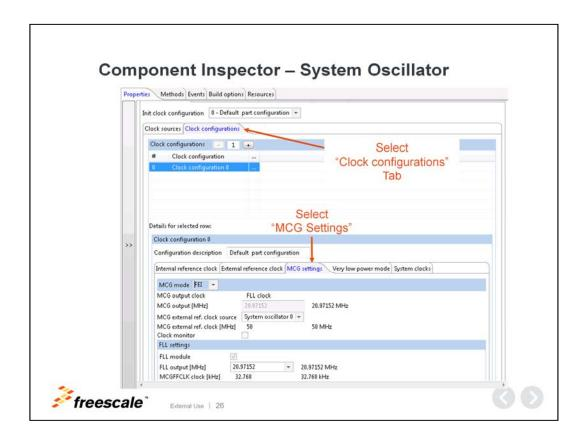
The input clock is set for 50MHz and now we will setup the clock configurations MCG
