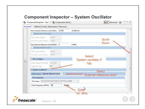
Based on the hardware design, the system has a 50MHz clock source, not a crystal.
