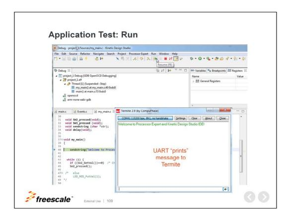
Notice the sendstring printed on the terminal and the green LED should be blinking.
