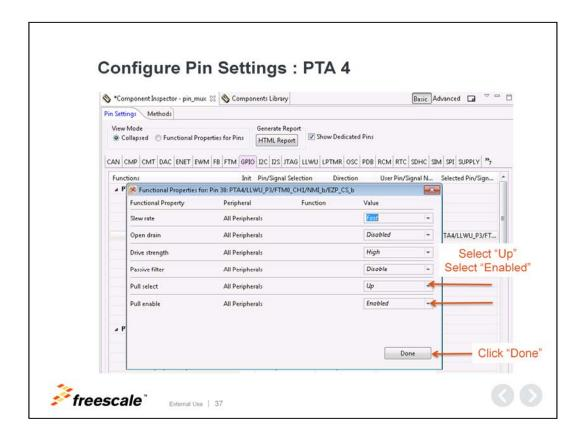
For the switch inputs, the switches require the use of the internal pull-up since there is no external pull-up on the schematic.
