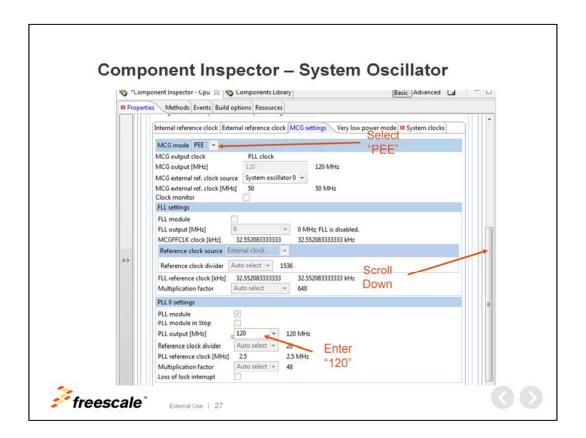
Here we are setting up the MCG. The board has an external 50MHz signal, and so to operate at maximum speed of the chip, the us of the PLL clock is required. So, select PEE, and set the PLL output to 120MHz.
