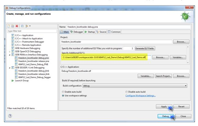
The **Debug session** will start and both the bootloader and demo application are now flashed on the MCU, you can now proceed to the section 3.1 "Debugging bootloader and demo application projects using the P&E interface".
