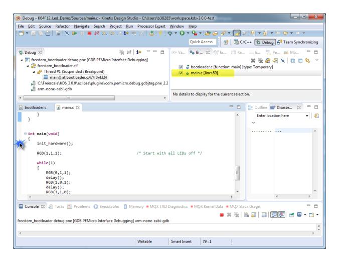
At this point you can step through the bootloader program and then jump to the demo application and continue debugging it:
