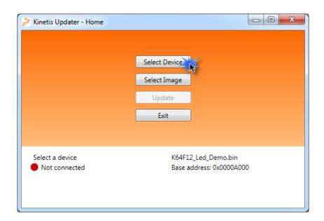
Select your device and click on **Connect**, if the connection is not established perform a reset to the board:
