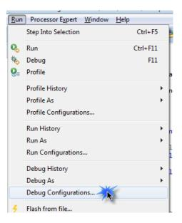
The debug configurations will open, choose the Segger interface and click on **Debug**. The same steps apply when using the P&E interface:
