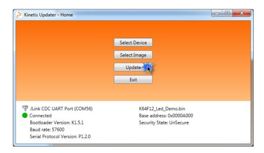
Click on the **Update** button and the application will be loaded to the MCU, the RGB led will start to toggle indicating that the bootloader jumped to the application:
