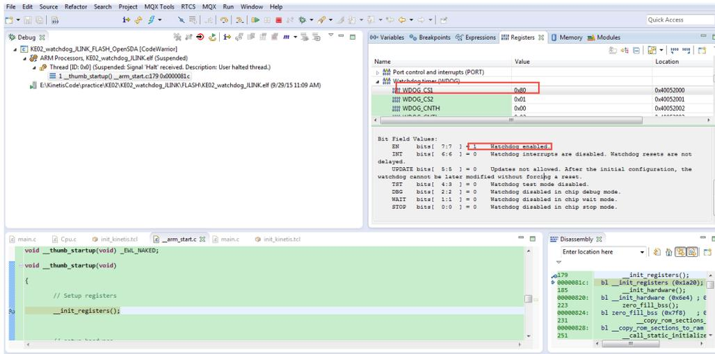
So, if you want to test the watchdog in debug mode, and want the EN is set after reset, you can choose PE debugger tool instead of JLINK, but this JLINK feature is just influence the debug mode, after you download the code to the chip flash, and after reset, the EN bit in WDOG\_S1 will still be set.
