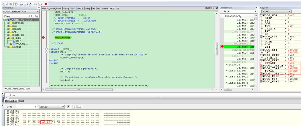
You can find, we need the TOVALL= 0XE8, TOVALH=0X03, but from the test result, the register is TOVALL= 0X03, TOVALH=0XE8, this will cause the timeout value is much larger than 1000, that is why customer can't reset the mcu after 1s, because the register configuration is not correct. It is caused by the IAR int16 store endian mode, the default IAR endian mode is little endian mode. So in the practical usage, it is recommended to use the separated time out value definition.
