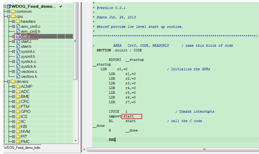
The above IAR start picture is for KE, but in the KEA start file, you can't see the start function in the KEA sample code which download from the freescale web, just find the \_\_iar\_program\_start in cstartup\_M\_KEA128.s after the reset happens, but where is the \_\_iar\_program\_start function, it can't be searched in the whole project. Actually \_\_iar\_program\_start is the default program entry function, it include the following function:
