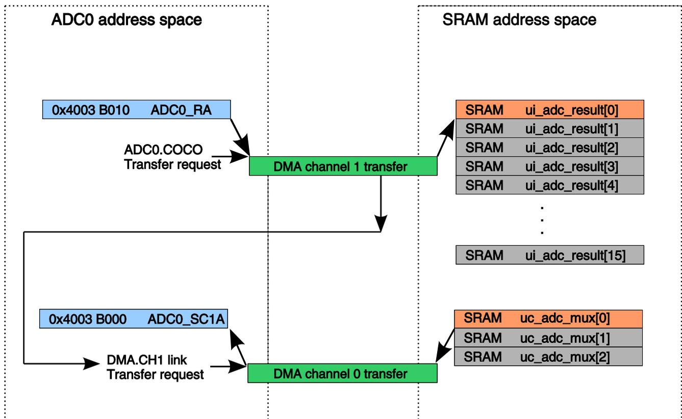
Figure 1. Data flow between periphery and SRAM
