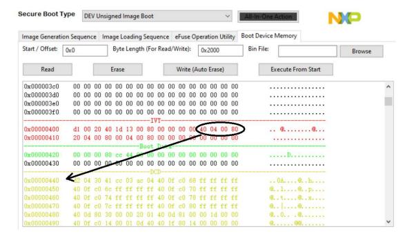
2. The IVT offset from the base address for each boot device type is defined in the table below. The location of the IVT is the only fixed requirement by the ROM. The remainder or the image memory map is flexible and is determined by the contents of the IVT.
