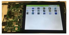
i. The debug terminal will indicate the boot progress as well. The login screen will indicate that the board has booted.
