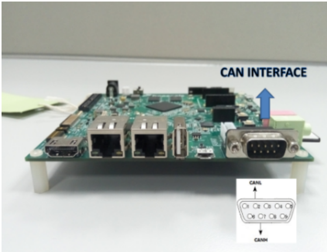
Figure 19.2.1: CAN bus interface DB-9 connector usage for i.MX 7Dual SDB board
