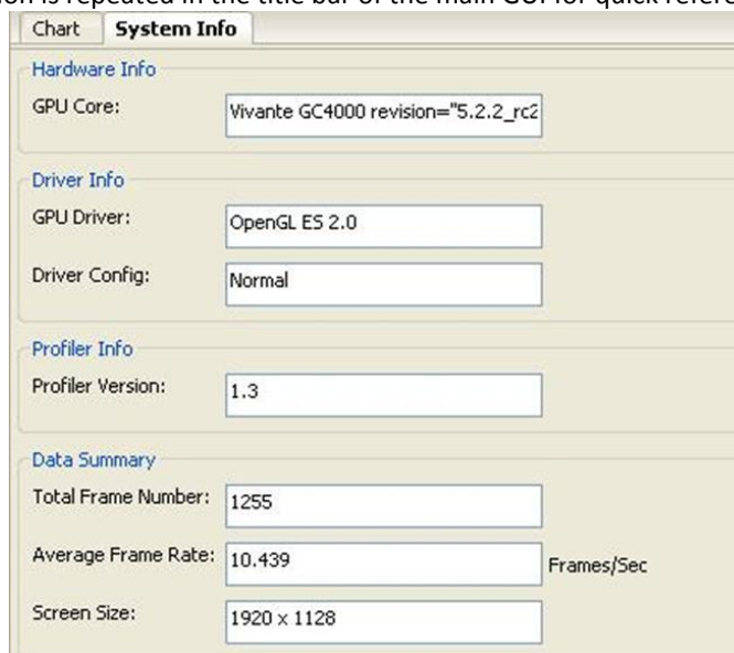
Figure 45 vAnalyzer System Info Tab
