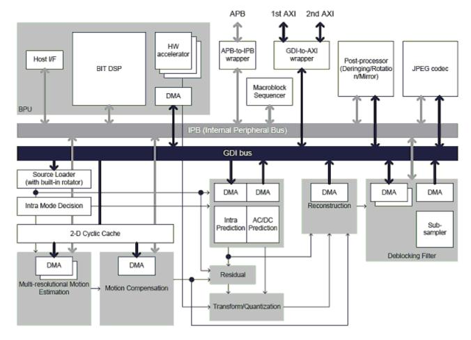
Figure 1. i.MX 6Dual/6Quad VPU Block Diagram
