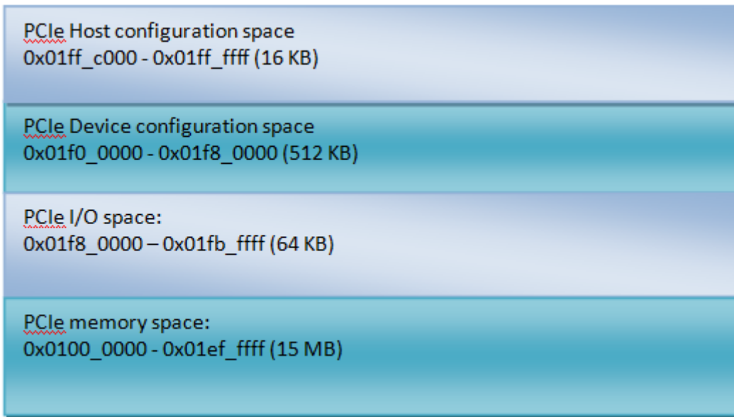
Figure 41-2. Memory Layout (i.MX 6Quad/6DualLite/6Solo)
