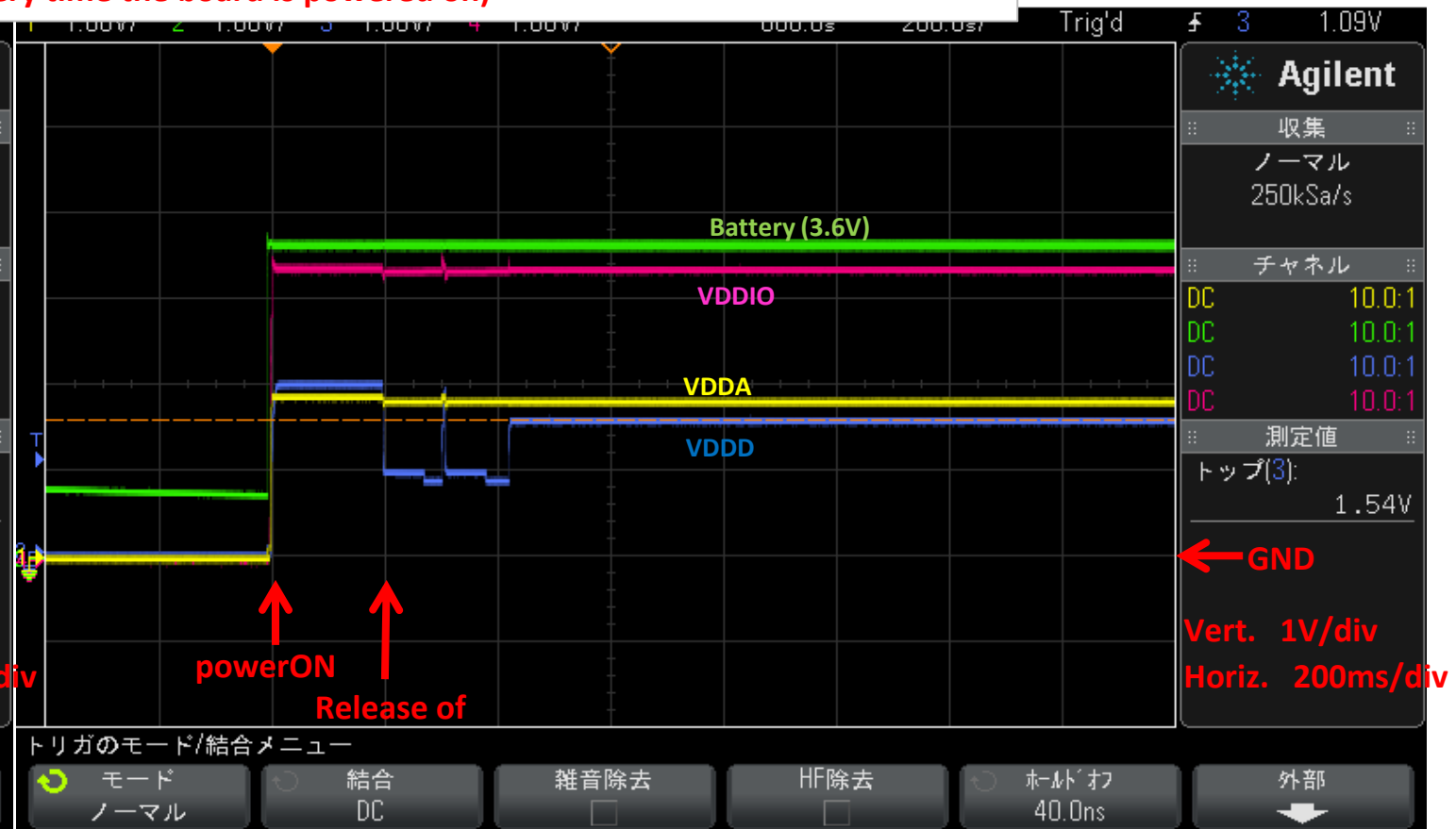
Power sequence of the Bad board (The waveform changes every time the board is powered on)
