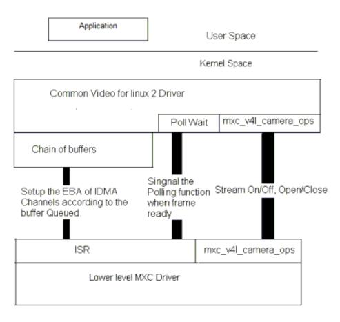
Figure 8-1. Video4Linux2 Capture API Interaction
