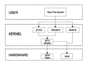
Figure 26-1. Components of a Flash-Based File System
