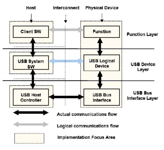
Figure 34-1. USB Block Diagram
