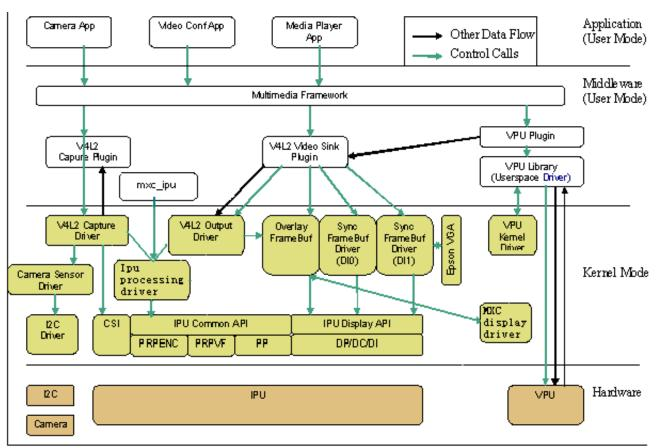
Figure 5-2. Graphics/Video Drivers Software Interaction for IPUv3
