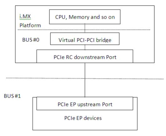
Figure 35-1. diagram of the PCIe RC port on i.MX 6
