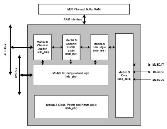
Figure 33-1. MLB Device Top-Level Block Diagram
