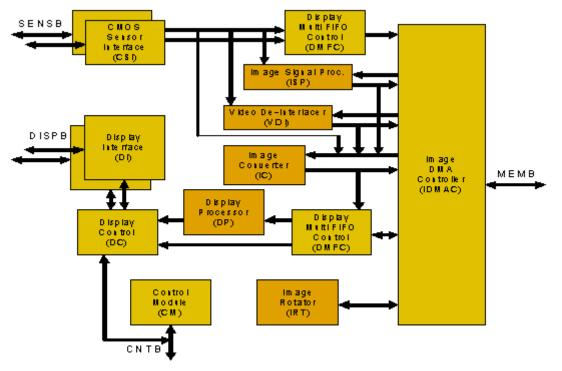
Figure 5-1. IPUv3EX/IPUv3H IPU Module Overview
