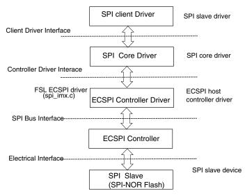
Figure 31-2. Layering of SPI Drivers in SPI Subsystem
