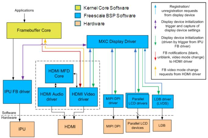
Figure 11-3. HDMI Video SW Architecture
