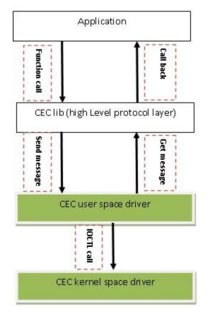
Figure 11-4. HDMI CEC SW Architecture
