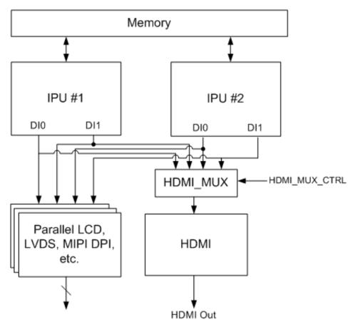
Figure 11-2. IPU-HDMI Hardware Interconnection
