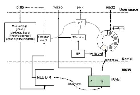
Figure 33-2. MLB Driver Architecture Diagram
