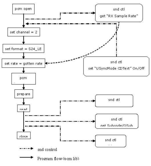
Figure 25-2. S/PDIF Rx Application Program Flow
