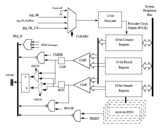
Figure 42-1. PWM Block Diagram
