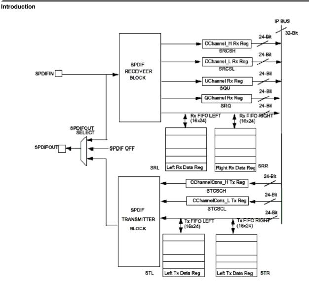
Figure 25-1. S/PDIF Transceiver Data Interface Block Diagram
