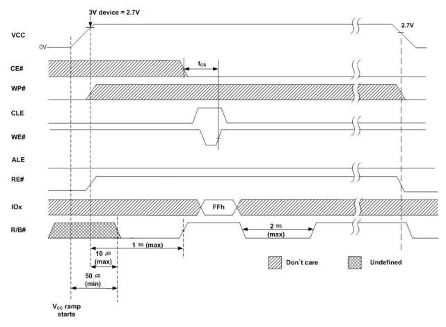
Figure 53 : Data protection and power on / off
