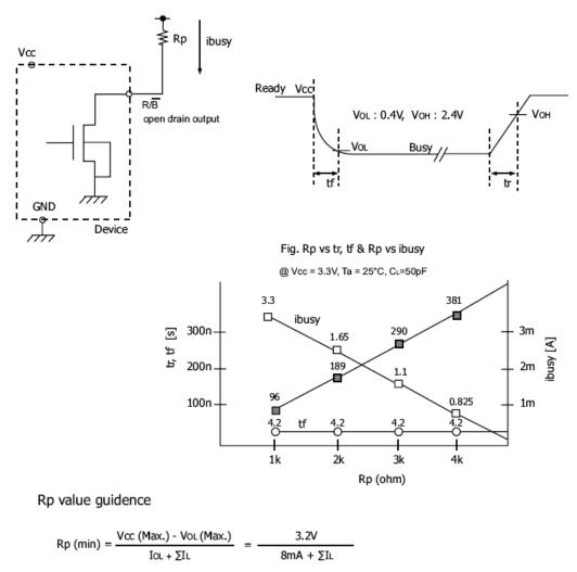
where IL is the sum of the input currnts of all devices tied to the  $R/\overline{B}$  pin. Rp(max) is determined by maximum permissible limit of tr
