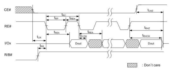
Figure 12 : Data output cycle timings (EDO)
