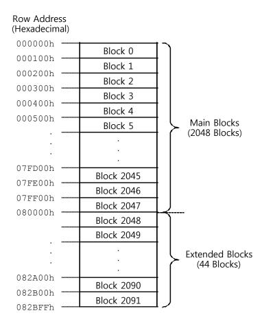
Figure 5 : Extended Blocks Arrangement
