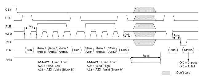
Figure 31 : Multi plane erase operation timings
