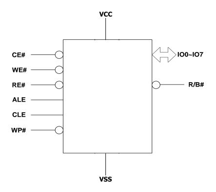
Figure 1 : Pin diagram(SDP)
