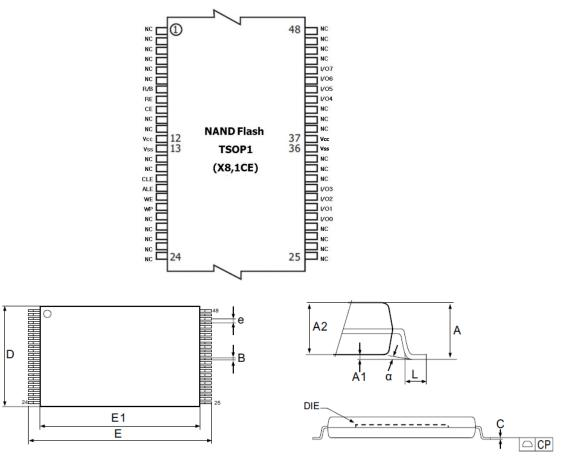
Figure 2 : 48-pin TSOP
