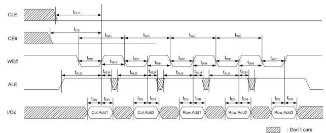
Figure 9 : Address latch timings
