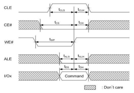
Figure 8 : Command latch timings
