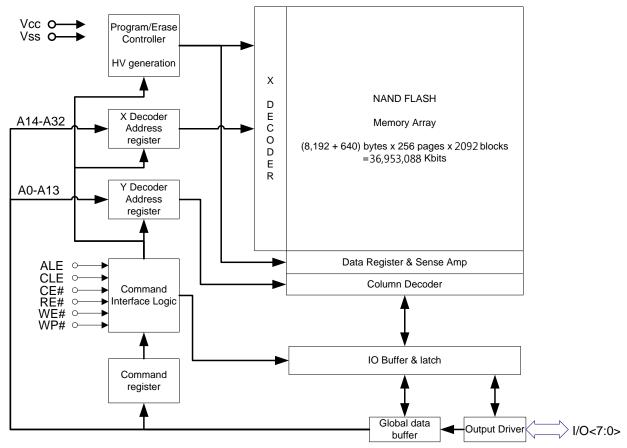
Figure 3 : Block diagram(SDP)
