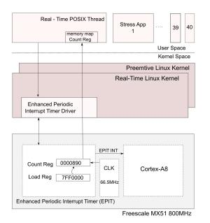
The tests were run for a day on a fully-loaded system collecting millions of samples. In order to load the system the "Stress" utility program was used. The Stress utility takes a number of parameters and loads the CPU, Input/Output, and the virtual memory.
