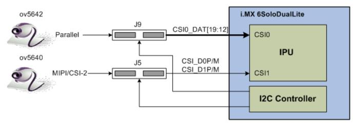
Figure 7-1. Camera Interface Layout
