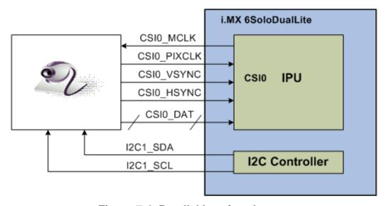
Figure 7-4. Parallel Interface Layout
