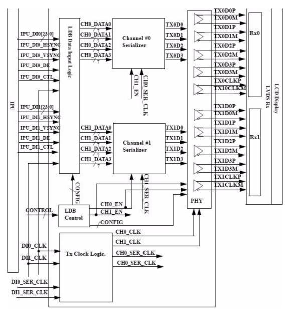
Figure 6-1. i.MX6 LVDS Display Bridge (LDB) Block
