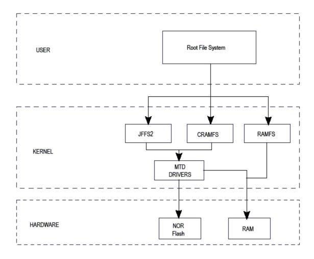
Figure 5-1. Components of a Flash-based file system
