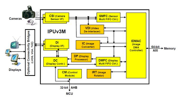
Figure 7-3. IPU Block Diagram
