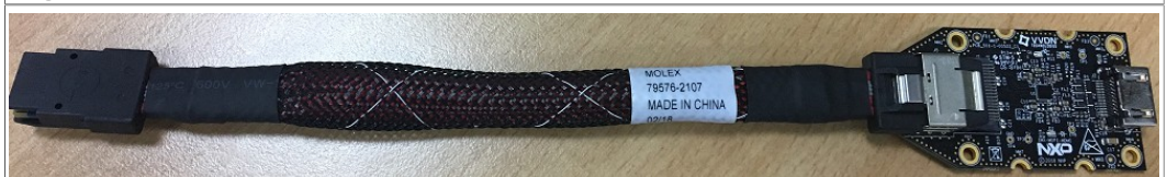
Figure 29. i.MX mini SAS cable with DSI-to-HDMI adapter
