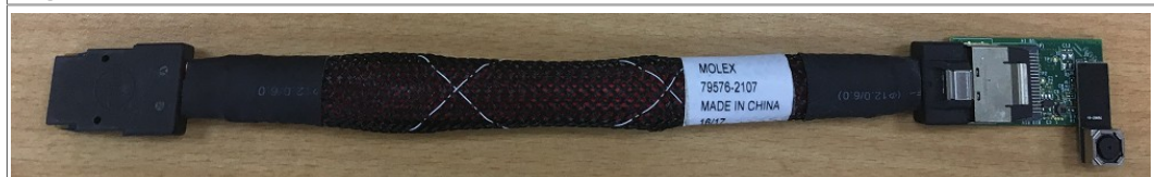
Figure 16. OV5640 CSI MIPI camera
