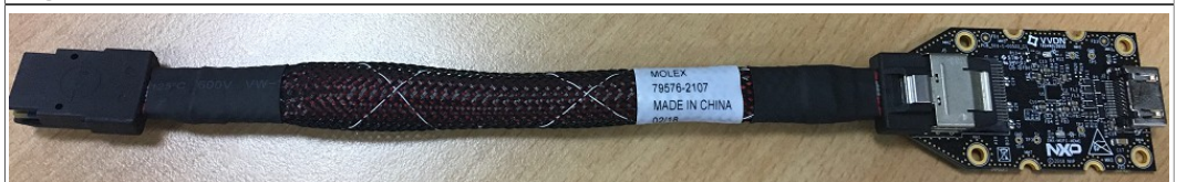
Figure 34. i.MX mini SAS cable with DSI-to-HDMI adapter
