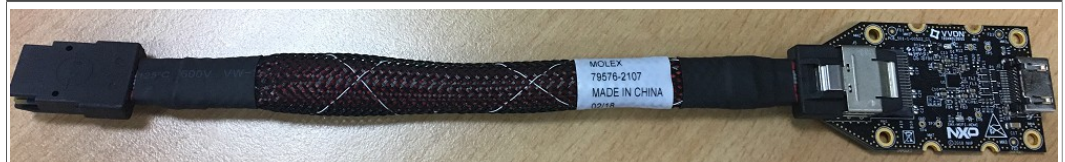
Figure 3. i.MX Mini SAS cable with DSI-to-HDMI adapter
