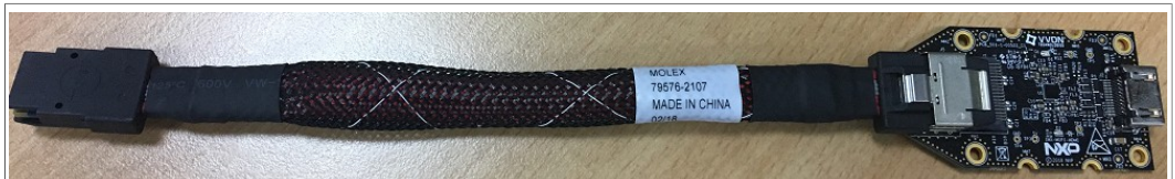
Figure 11. i.MX mini SAS cable with DSI-to-HDMI adapter
