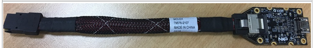
Figure 21. i.MX mini SAS cable with DSI-to-HDMI adapter
