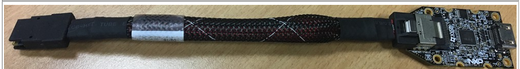
Figure 35. i.MX mini SAS cable with LVDS-to-HDMI adapter
