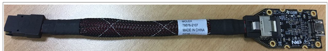
Figure 7. i.MX mini SAS cable with DSI-to-HDMI adapter
