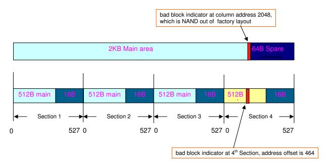
Here is the summery of the incompatibility between the NAND flash layout and the FSL NFC data layout:
