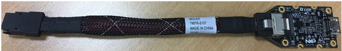
Figure 3. i.MX 8M Mini SAS cable with DSI-to-HDMI adapter
