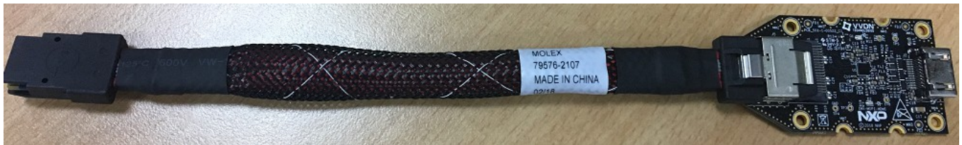
Figure 9. i.MX mini SAS cable with DSI-to-HDMI adapter
