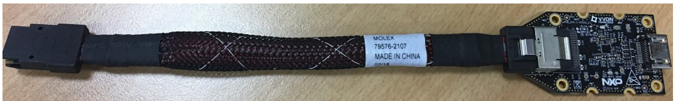
Figure 20. i.MX mini SAS cable with DSI-to-HDMI adapter
