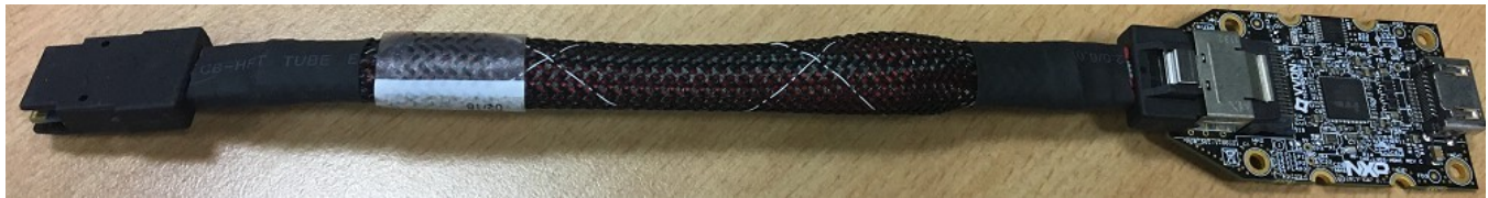
Figure 21. i.MX mini SAS cable with LVDS-to-HDMI adapter
