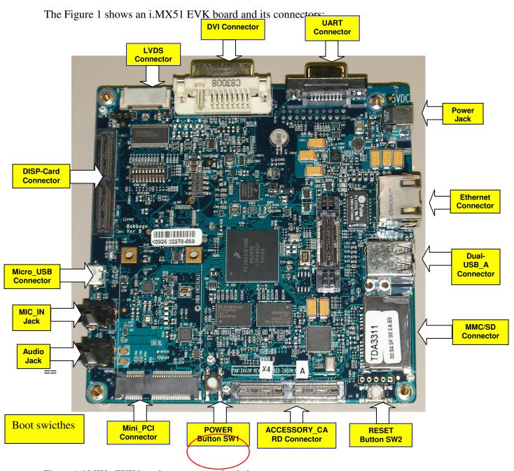
Figure 1: i.MX5. EVK board connectors and switches
