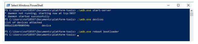
Note to see if your board successfully entered to Bootloader mode. In your serial terminal, you should see that you are in Bootloader mode.
