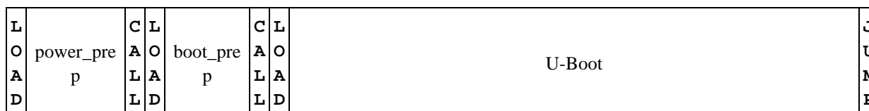
Figure 1-3 An example of i.MX23 Boot stream loading U-Boot
