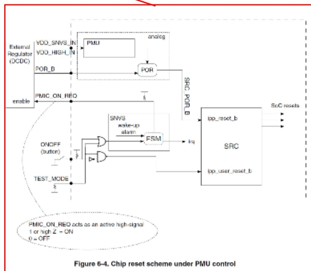
Figure 6-4. Chip reset scheme under PMU control
