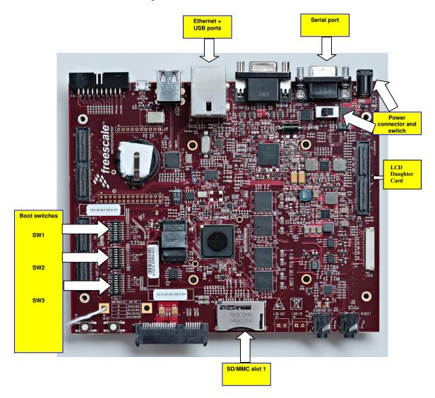
Figure above takes MX53 EVK RevA board (Red color) as the example. MX53 EVK RevB board (Blue color) is similar to RevA board. Please refer to Hardware documentation to know the detailed difference between RevA and RevB boards.
