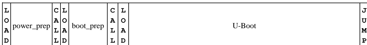
Figure 1-3. Example of i.MX28 Boot Stream Loading U-Boot
