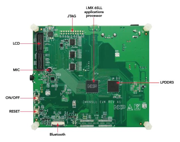
Figure 3. Back side of i.MX 6SLL EVK (bottom)
